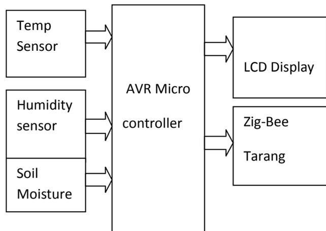
5. Block diagram of Transmitter
