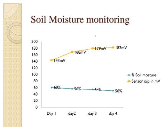
Figure 10 soil moisture monitoring in Feb2014
