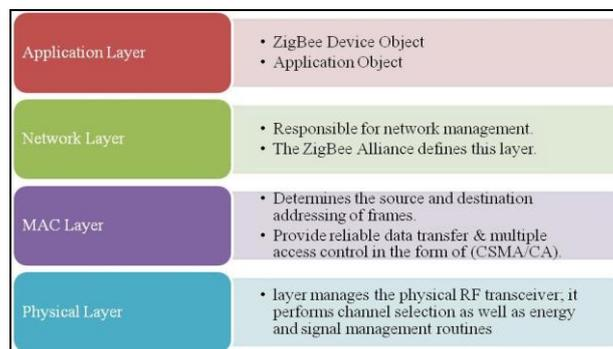
Fig.1 ZigBee Layers
