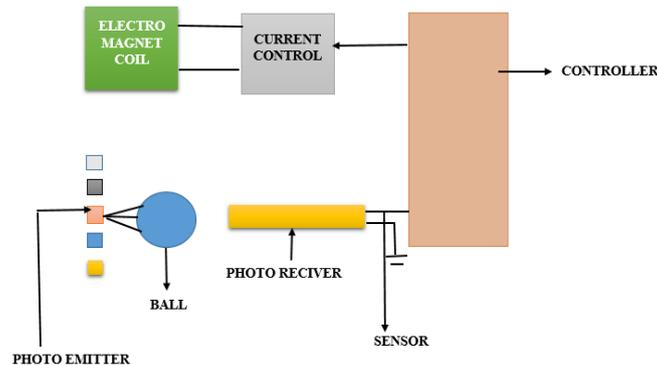
Fig 2. Schematic diagram of magnetic levitation<sup>[14]</sup>
