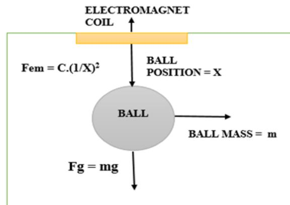
Fig 3: Magnetic Levitation with free body diagram[14]
