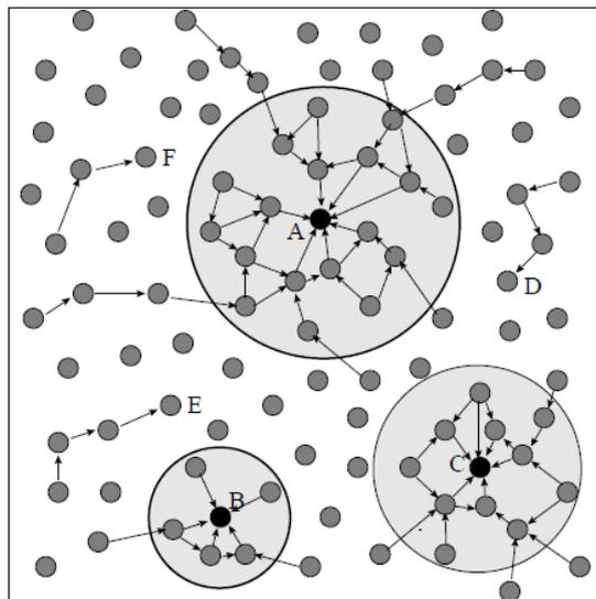
Fig. 4 Proactive zones of node A, B, C in SHARP [13]
