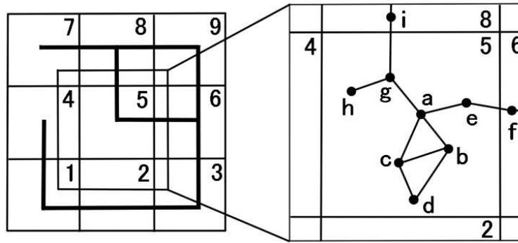
Fig. 5 Zone and Node Topology in ZHLS [15]
