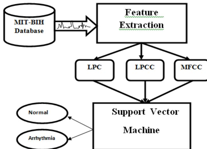
Fig.1. Block Diagram of ECG classification
