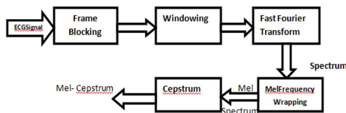
Fig.5. Block Diagram of MFCC computation
