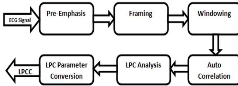
Fig.3. Block Diagram of LPC Computation
