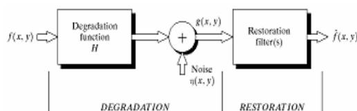
Figure1: A Model of the degraded/restoration process
