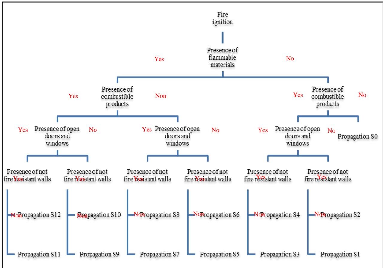
Fig. 1: Event tree describing all cases of fire spreading in a building
