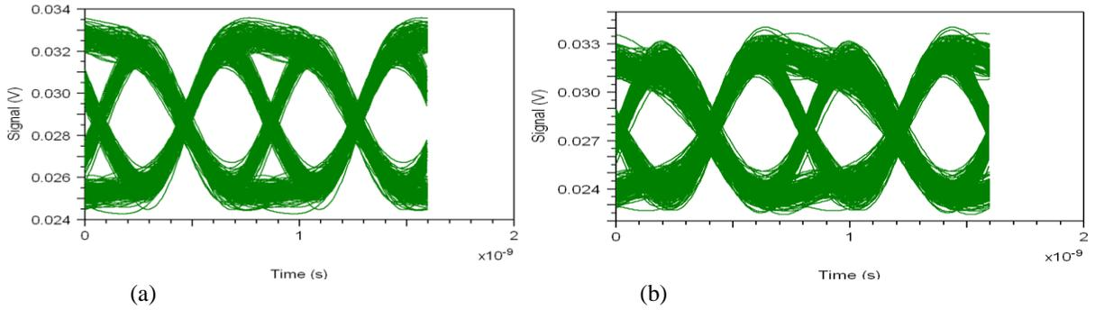
**Fig4.** Eye diagrams of hybrid passive optical network system using 320 users with Manchester modulation format at (a) 110, (b) 160 km distance respectively.
