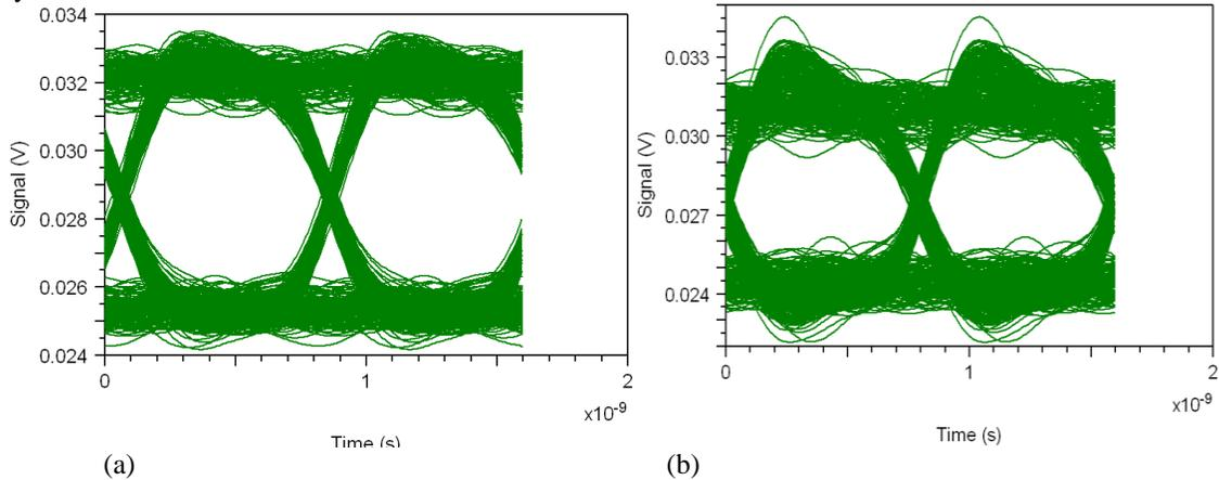
**Fig3** Eye diagrams of hybrid passive optical network system using 320 users with NRZ modulation format at (a) 110, (b) 160 km distance respectively
