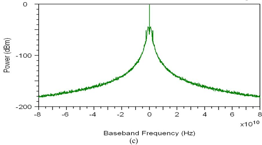
Fig 5 .Baseband signal spectrum (a) for RZ (b) for NRZ (c) for Manchester modulation format.
