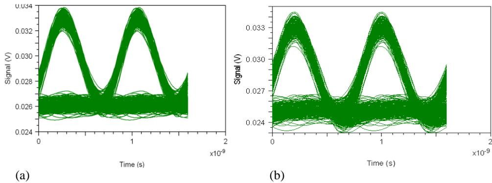
**Fig2.** (a)–(b)Eye diagrams of hybrid passive optical network system using 320 users with RZ modulation format at (a) 110 (b)160 km distance respectively.
