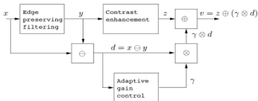
Fig. 2. Block diagram of the proposed generalized unsharp masking algorithm.
