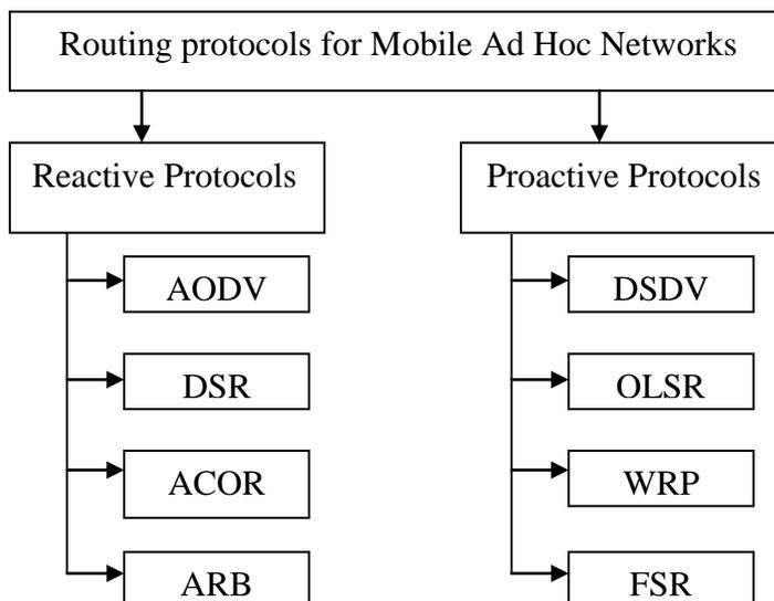
Fig. 1 Classification of routing protocols
