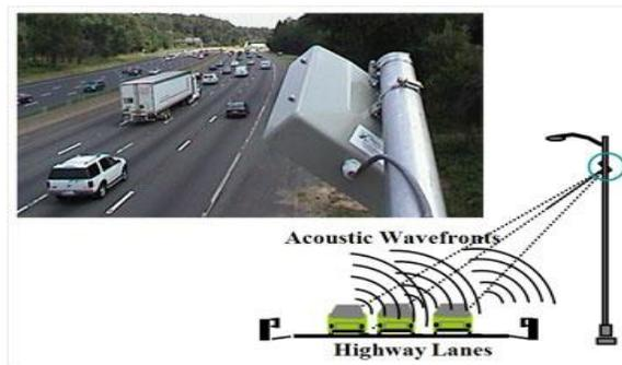
Fig10: Passive Acoustic Detectors Transportation Control Systems' Products Details [22].
