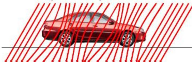
Fig2 - Earth's Magnetic Field through Vehicle [2].
