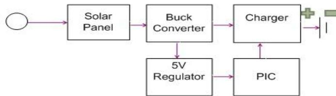
Fig 2:Block Diagram Solar Charging
