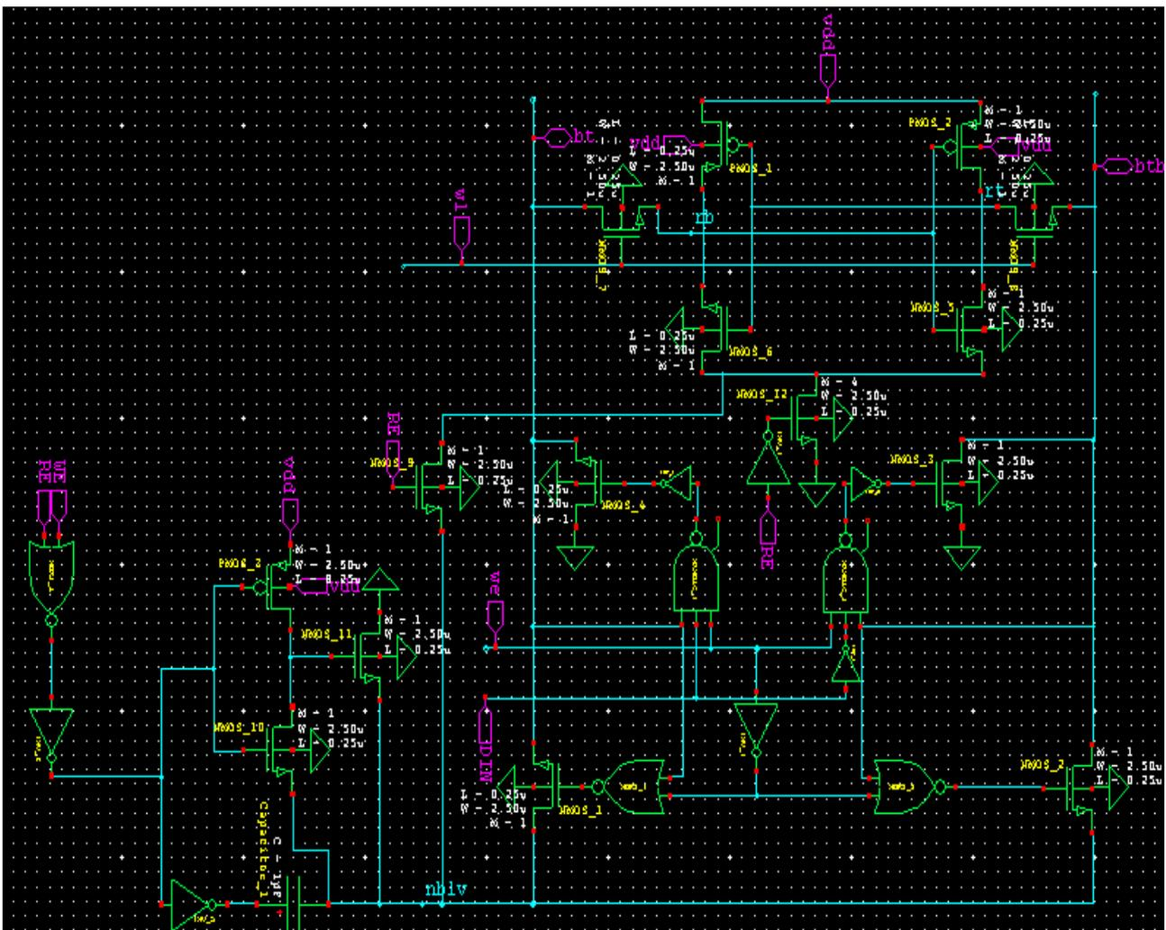
Fig 3 Schematic of the proposed common write and read assist circuit [29] in tanner tool
