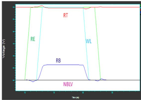
Fig 4 Successful read operation without proposed circuit [29]
