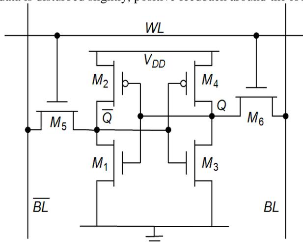
Figure 1 Six-transistor SRAM cell
