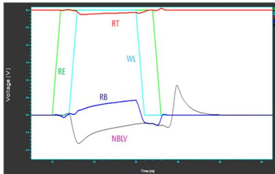
Fig 5 Successful read operation with proposed circuit [29]
