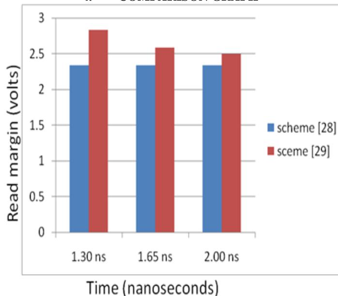
Fig 6 Comparison of read margins between scheme [28] and proposed scheme [29]
