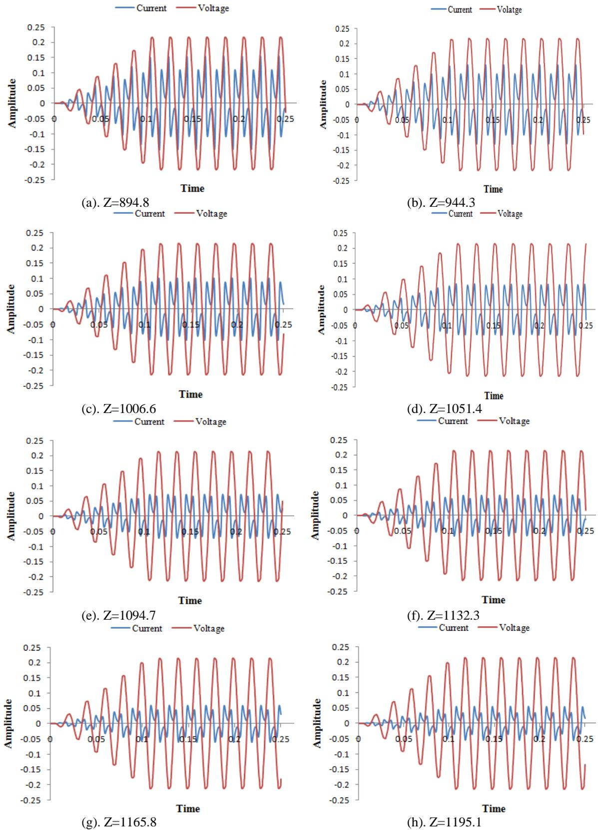
Fig. 3(a-h) Signal for output current and voltage are recorded at 16,000 sampling rate for eight different values of inductance, keeping resistance (124Ω) and capacitor (2.5μF) are constant
