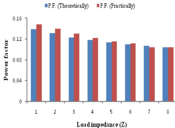
Fig. 4 Calculated theoretical and practical value of power factor for different impedance value
