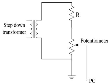
Fig. 2 Voltage step-down circuit to input signal to PC
