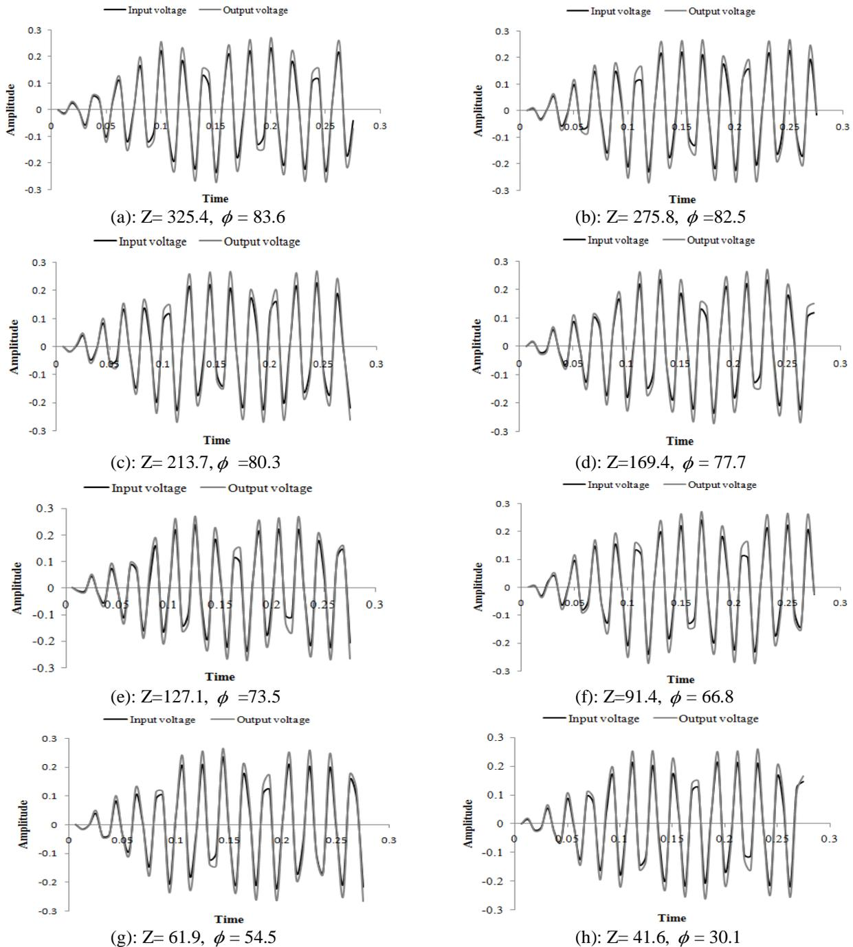
Figure 3(a-h): Input and output voltage signals with eight varying values of inductance and constant values of resistance and capacitance for duration 0.26second
