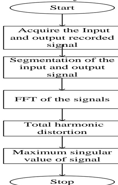
Figure 2: Algorithm flow chart to calculate input and output signal of THD
