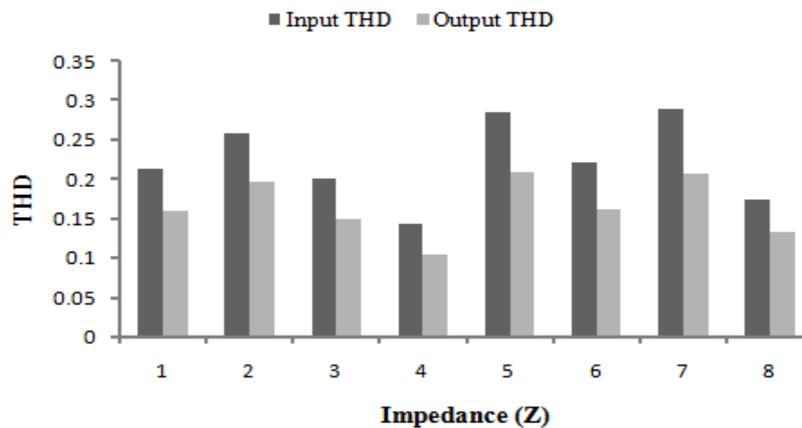
Figure 4: Calculated value of input and output THD with different of impedance value
