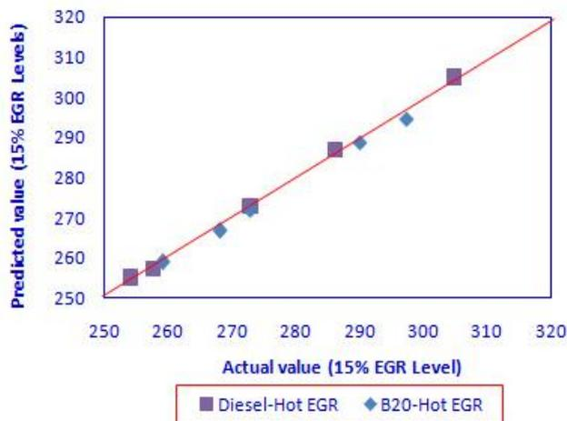
Fig 4. Actual Vs Predicted with 15% hot EGR in Head position
