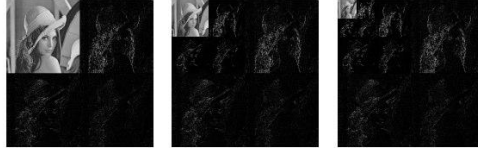
Figure 2.5: Pyramidal decomposition of Lena image (1, 2 and 3 times)
