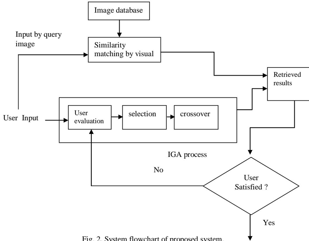
Fig. 2. System flowchart of proposed system.
