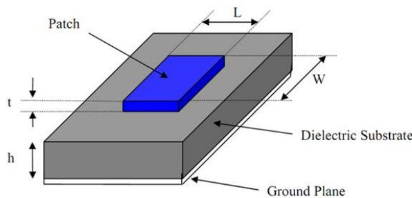
Fig 1. Basic Structure of a Microstrip Antenna
