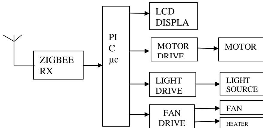
Fig. 3 Block Diagram of Receiver
