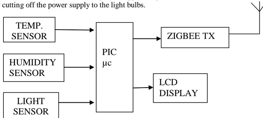
Fig. 2 Block Diagram of Transmitter
