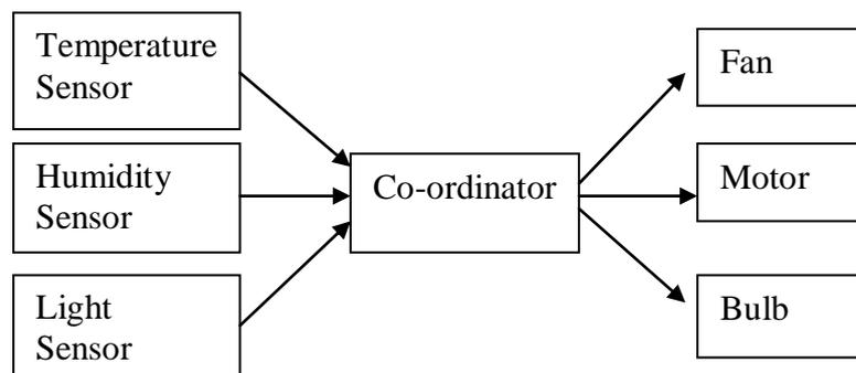
Fig. 1 Star Network Applied in Polyhouse.
