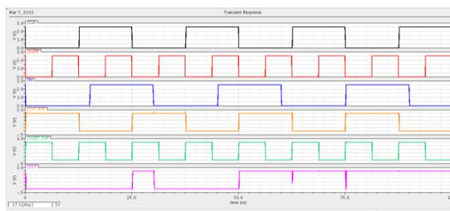
Fig. 9. Waveforms of MTCMOS latch circuit.
