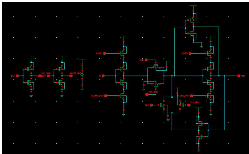
Fig. 3. MTCMOS latch circuit.
