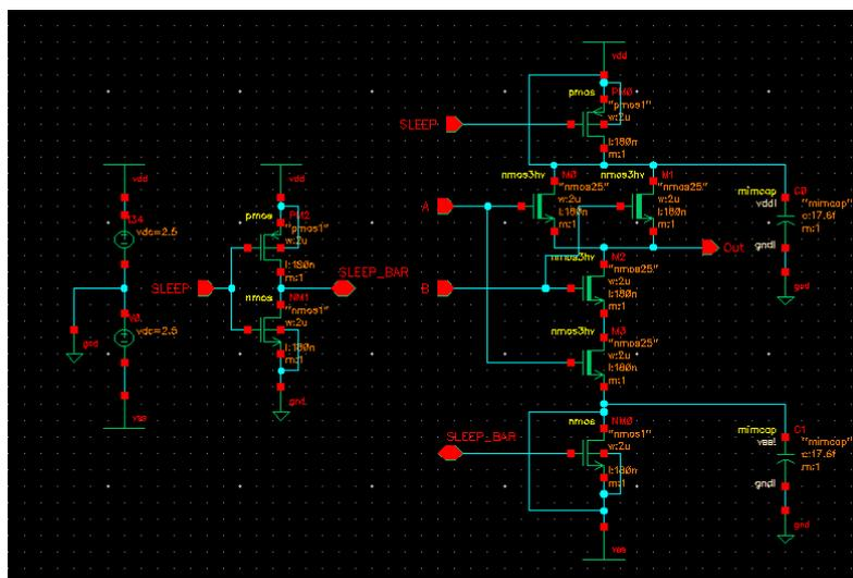
Fig. 2. MTCMOS circuit scheme.
