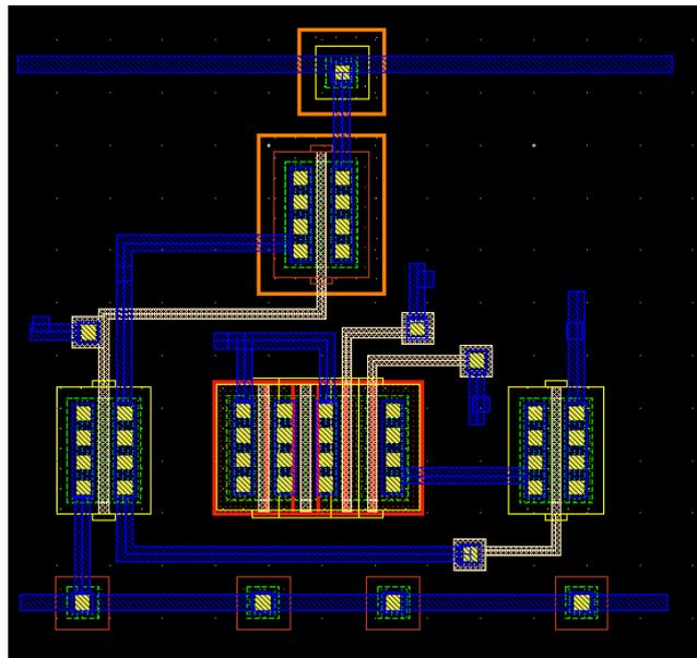
Fig. 7. Layout of MTCMOS circuit scheme B.
