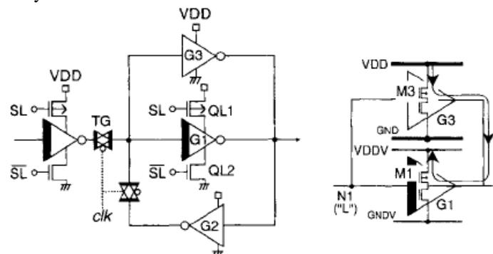
Fig. 2. MTCMOS Latch circuit.
