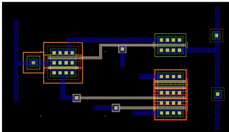
Fig. 6. Layout of MTCMOS circuit scheme.
