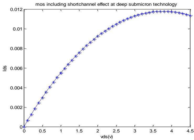
Fig.17 Shows drain-current voltage characteristics at deep submicron technology (.35 um) including short channel effect. The value of current decrease due to short channel effect.
