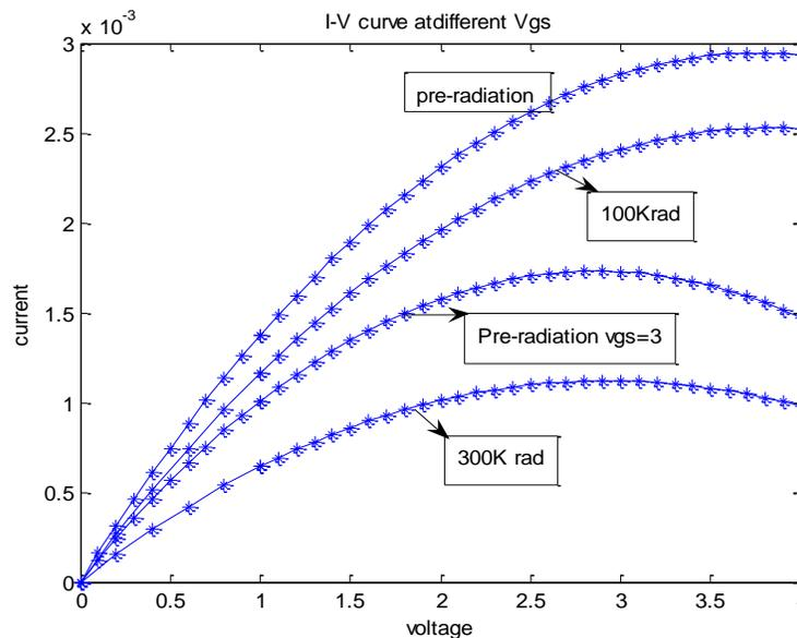
Fig.20 Shows effect of radiation on  $I_{ds}$ - $V_{ds}$  curve. Current decreases with increasing dose.
