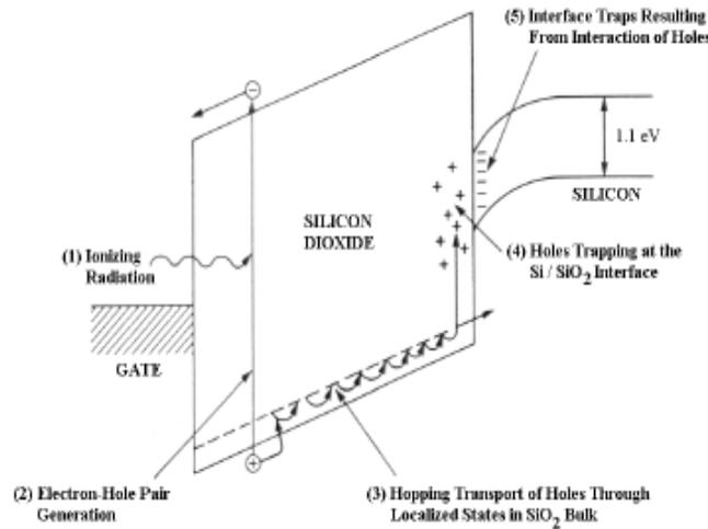
Fig.2: Schematic illustration of the effects induced by ionizing radiation in an MOS device [7]
