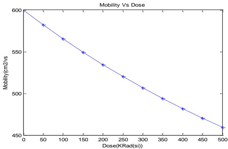
Fig.17 MOSFET mobility reduces with the increase in dose (Krad).
