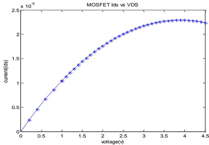
Fig.13 Shows  $I_{ds}$  vs.  $V_{ds}$  MOSFET characteristics with short channel effects and radiation effects.
