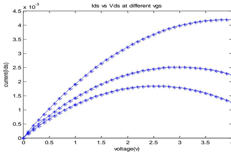
Fig.14 shows Drain-Current voltage characteristics at different  $V_{gs}$  4V, 3V, 2.5V at 1  $\mu$ m technology including short channel effects
