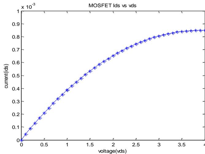
**Fig.11** Variation in Ids and Vds at Constat  $V_{gs}=4.0$  V including channel length modulation.This graph shows that Ids increases due to channel length modulation.
