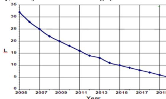
**Fig.5** Gate length (in micron) scaling [1]
