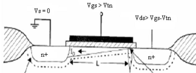
Fig.8 Channel length modulation
