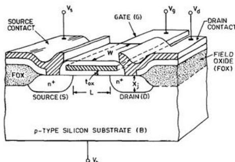
Fig.1 Schematic diagram of a MOSFET [2]
