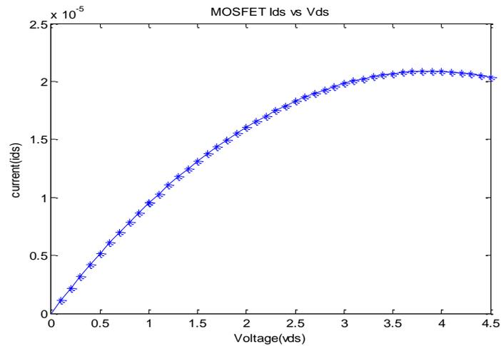
**Fig.10** Variation of Ids and Vds at Constat  $V_{gs}=4.0$ V including mobility degradation.This graph shows Ids reduction due to mobility degradation.
