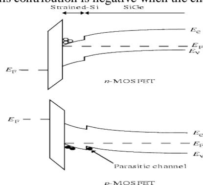
Fig.3 Energy bands diagrams in the silicon for an n-channel and a p-channel transistors [7]
