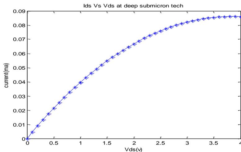
Fig.15 shows drain-current voltage characteristics at deep submicron technology. The value of current increases in deep submicron technology.
