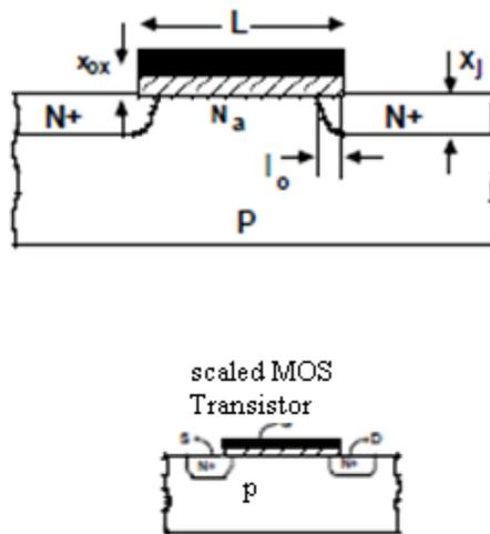
Fig.6 Shows MOSFET Device Scaling [1]
