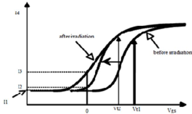
**Fig.4:** Increase of the sub-threshold current in a n-channel transistor given by a decrease in the threshold voltage and in the sub -threshold slope [3].
