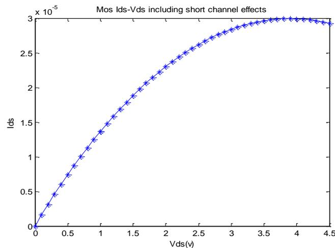
**Fig.12** Shows Ids vs. Vds curve including short channel effects. This curve depicts that by including short channel effects drain current decreases.
