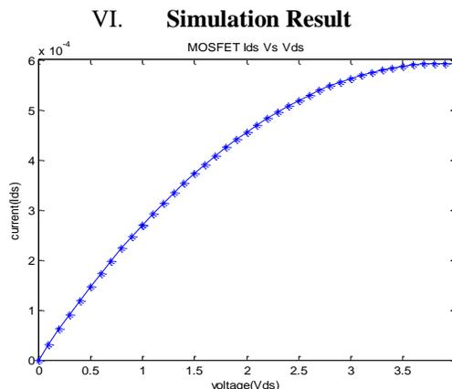
**Fig.9** this waveform shows variation in  $I_{ds}$  vs.  $V_{ds}$  at constant  $V_{gs}=4.0$  V
