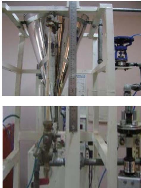
Fig 1: Real experimental setup of the conical tank process
