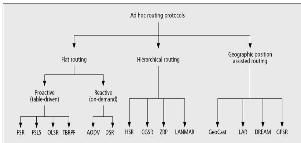
Fig. 1 Classification of Routing Protocols in MANETs
