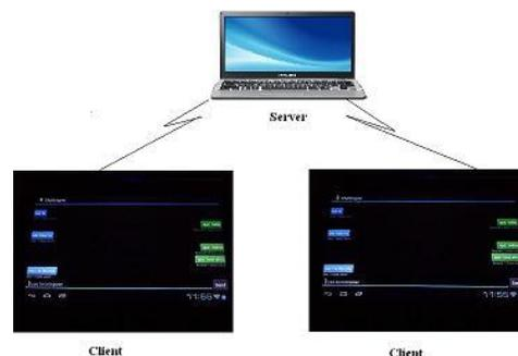
Figure 3.4 Message transfer between android devices (Aakash Tablets) via intranet server using Wi-Fi.
