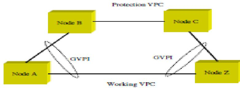
Fig 1: Working and protection VPCs
