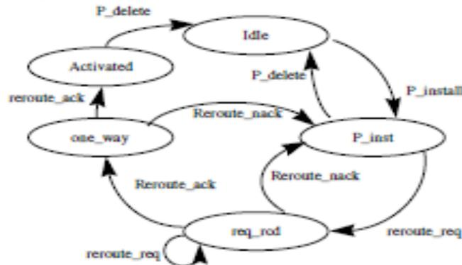
Fig. 3: Connecting point node state diagram
