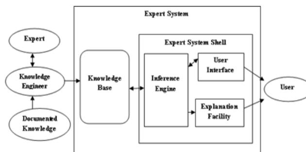
Fig. 1 Expert system Architecture
