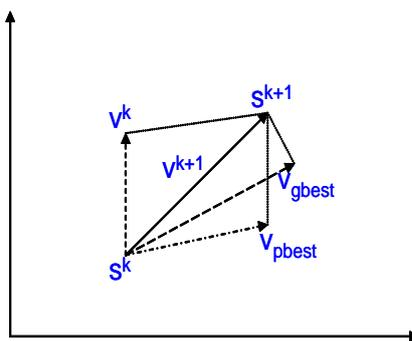
Fig.2 Concept of modification of a searching point by PSO
