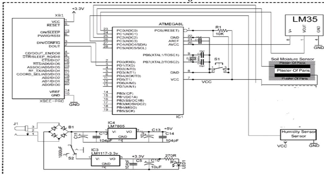
Figure.4 Circuit Diagram of Transmitter
