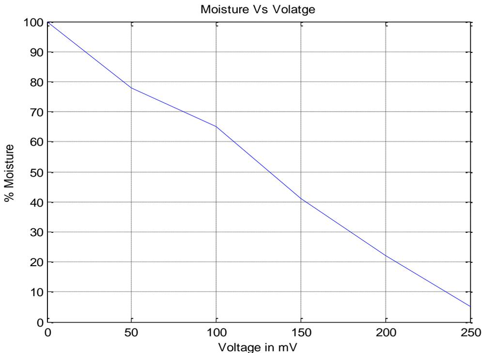
Figure.8 Response of moisture sensor
