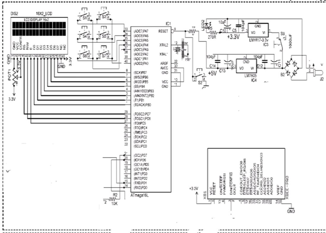
Figure.5 Circuit Diagram of Receiver
