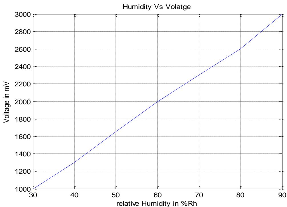
Figure.9 Response of humidity sensor
