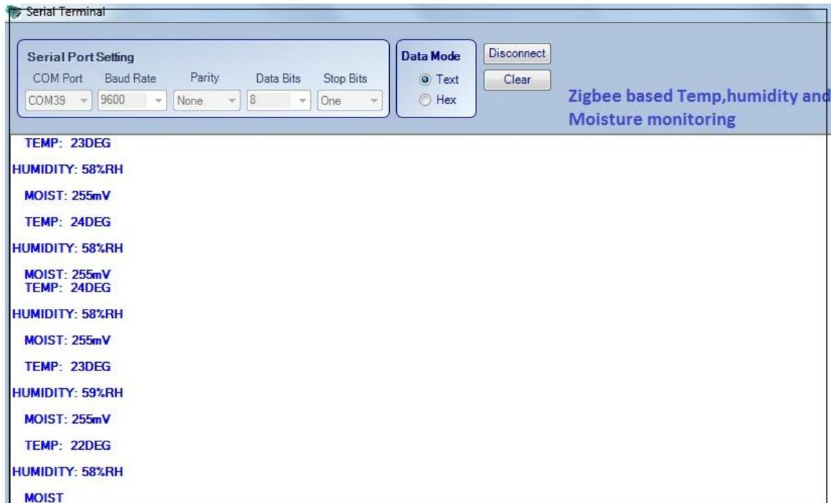
Figure.11 All parameter monitoring on computer using serial port
