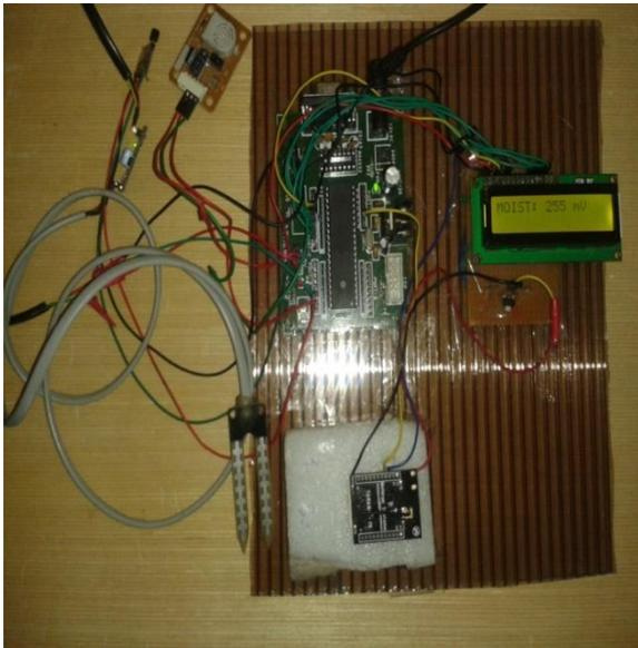
Figure.6 Prototype of Transmitter
