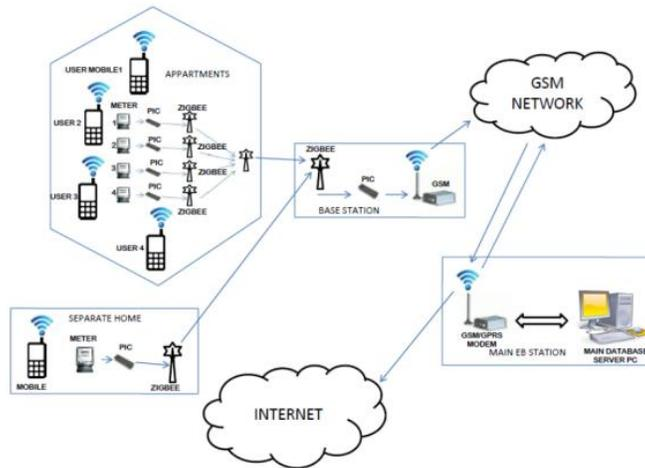
Fig 1: Architecture of monitoring system
