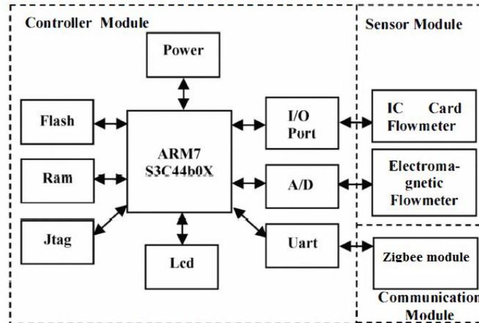
Fig 2: Hardware for monitoring point
