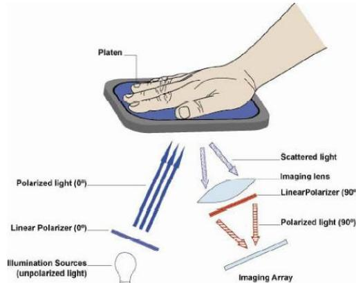
Figure1: Major optical components and layout of the hand imaging system
