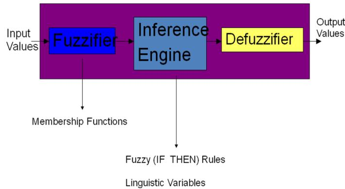
Fig 2: Block diagram of Fuzzy logic controller
