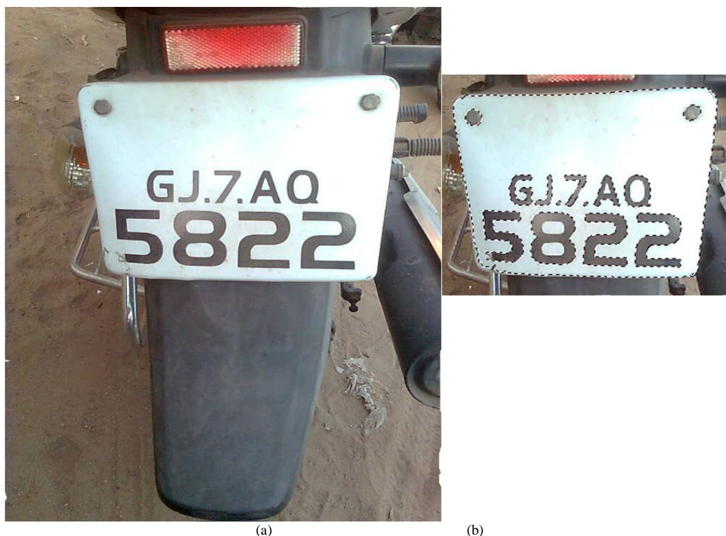
Fig. 2. (a) Image of vehicle (b) Image of vehicle number plate after image segmentation
