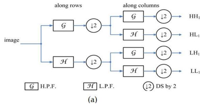
Figure 1.6: Wavelet decomposition of an image.
