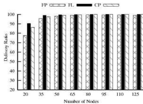
Fig. 10: Host density vs delivery ratio in static network i.e. mobility speed = 0m/s
