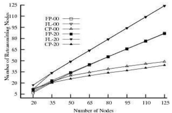
Fig.12: Host density vs. number of retransmitting nodes in static and dynamic network
