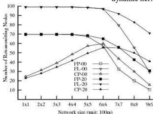
Fig. 8: Network size vs number of retransmitting nodes in static and dynamic network
