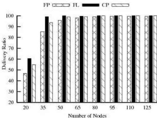
Fig. 11: Host density vs delivery ratio in dynamic network i.e. mobility speed = 20m/s
