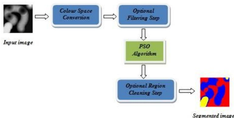
Fig 1: PSO Based Image Segmentation of a synthetic image.
