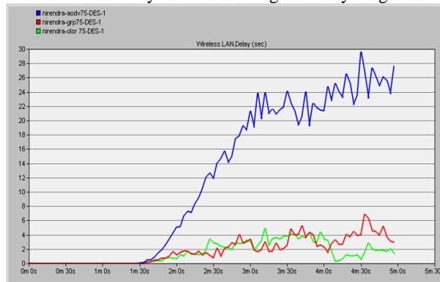
Fig. 1.1: Delay Comparison in Three Routing Protocols with 75 Nodes
