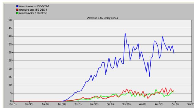
Fig. 1.2: Delay Comparison in Three Routing Protocols with 150 Nodes
