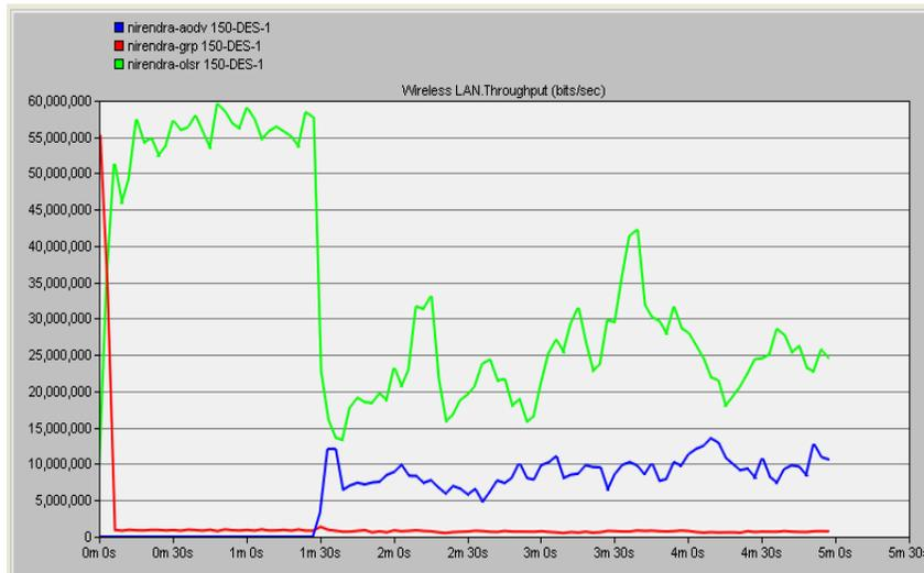
**Fig. 1.4:** Throughput (bits/sec) Comparison in Routing Protocols with 150 Nodes
