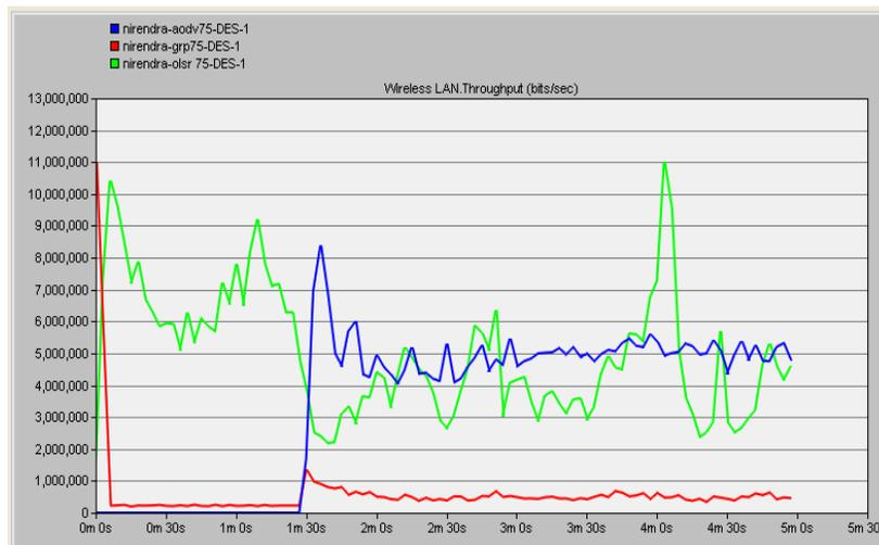
**Fig. 1.3:** Throughput (bits/sec) Comparison in Routing Protocols with 75 Nodes
