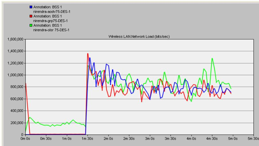
**Fig. 1.5:** Network Load (bits/sec) Comparison in Three Routing Protocol with 75 Nodes
