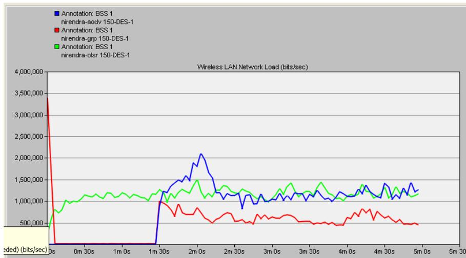
**Fig. 1.6:** Network Load (bits/sec) Comparison in Three Routing Protocol with 150 Nodes
