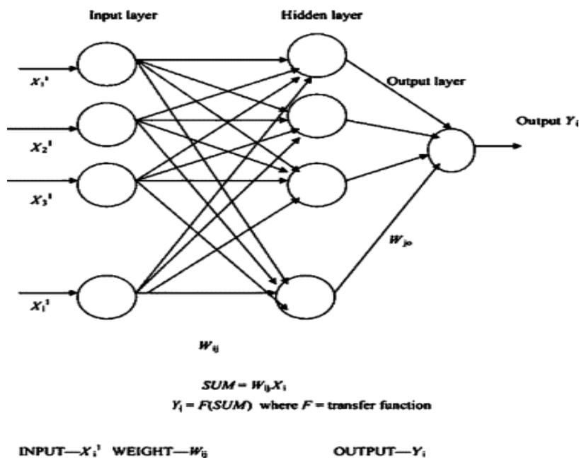
Fig. 2 The basic architecture of multilayered ANN
