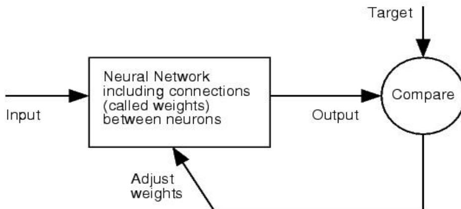
Fig. 3 Back Propagation of multilayered ANN
