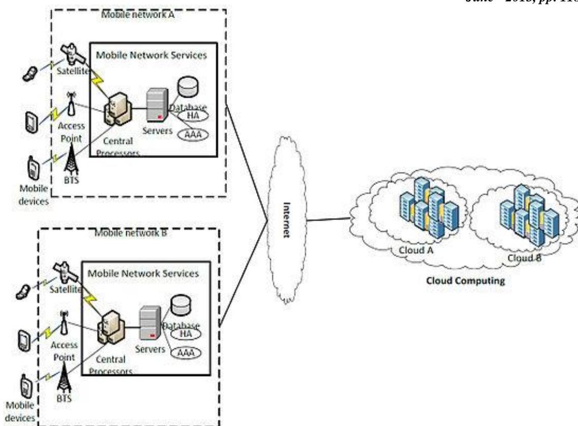
Fig. 2 Architecture of Mobile Cloud Computing
