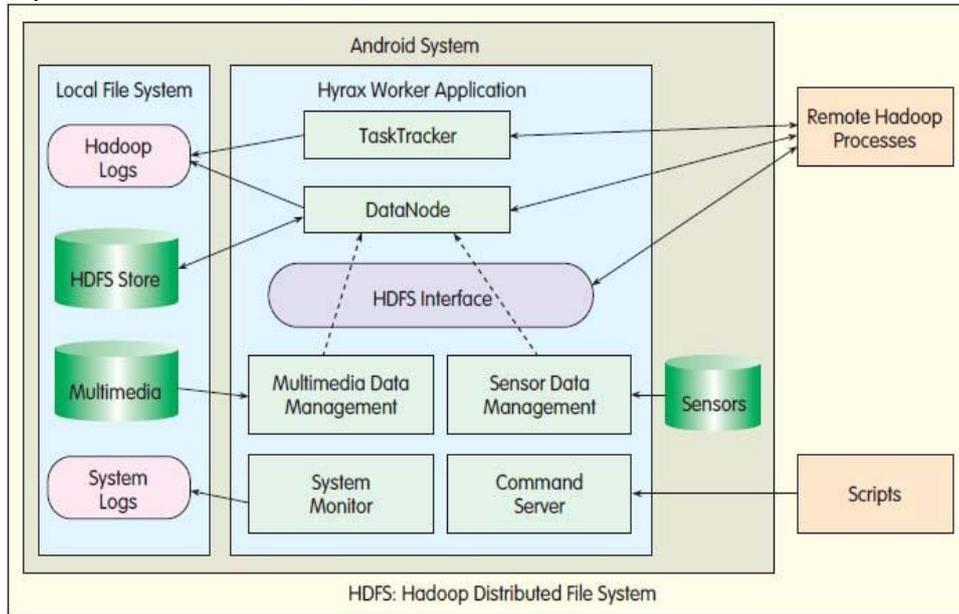
Fig. 3 Hyrax worker application component interaction diagram.
