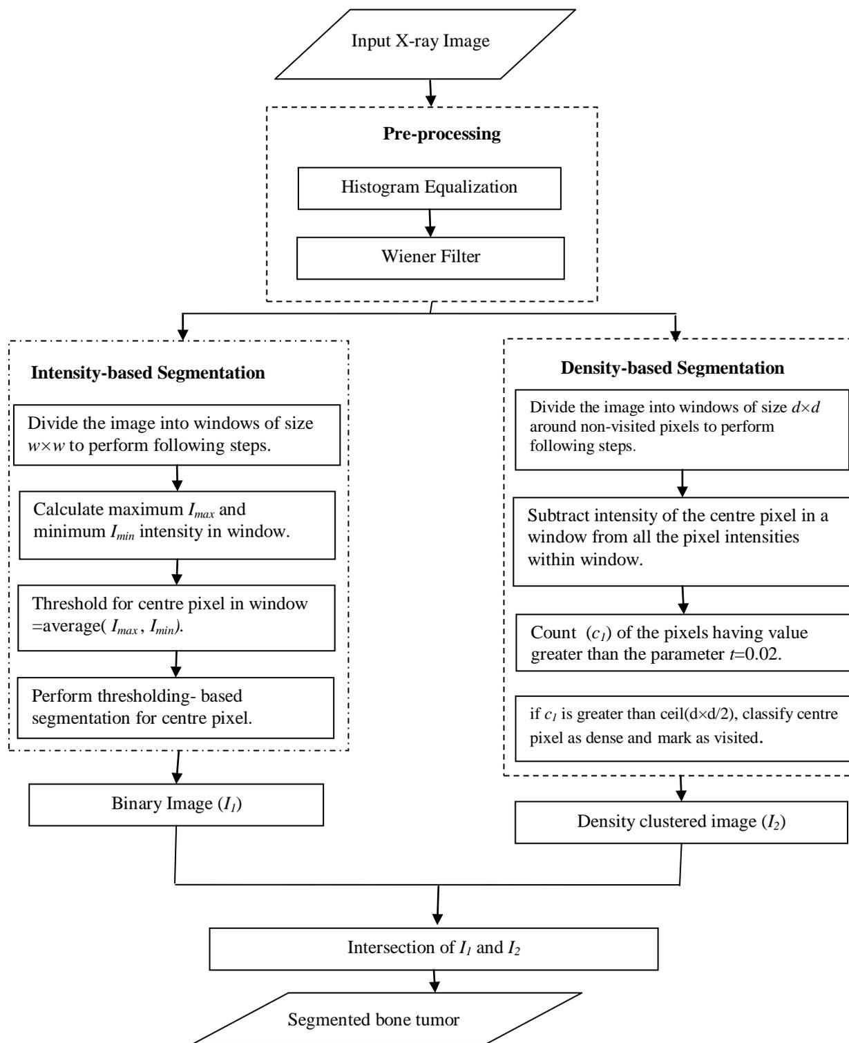
Figure 1: Architecture of the proposed method.
