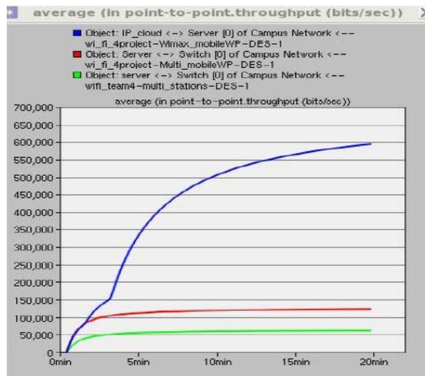
Figure 12: Throughput of the inward link to the server.
