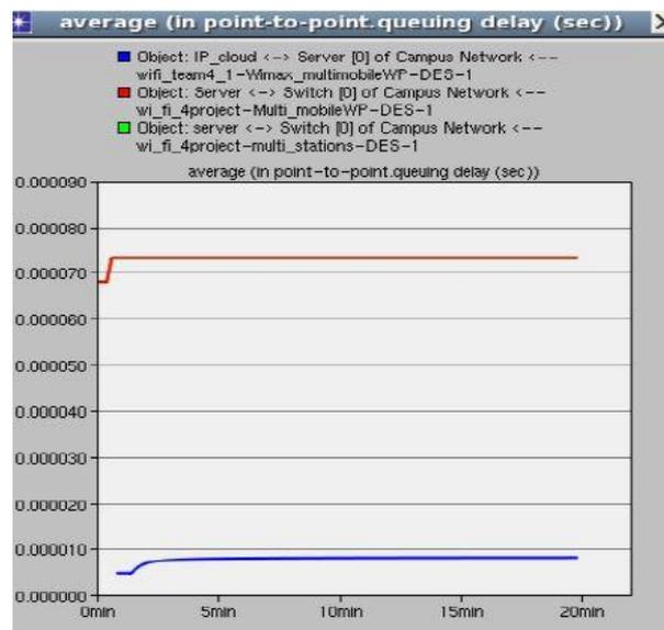
Figure 15: Average queuing delay of the server to switch link in WiFi and the IP cloud to server link in WiMAX.
