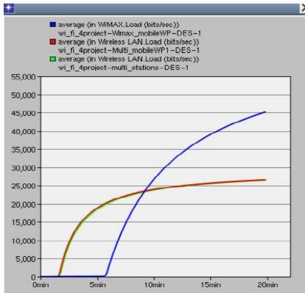
Figure 14: Load of BS and access point.
