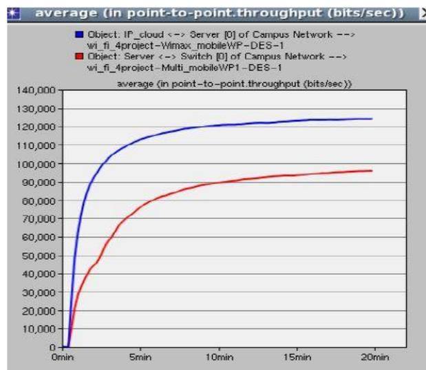
Figure 13: Throughput of the outward link from the server.
