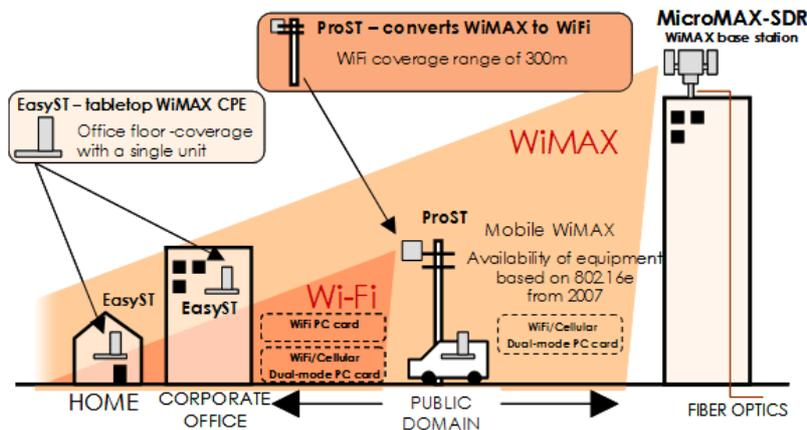
Figure 3: WiFi and WiMAX client/station connections to the Internet.
