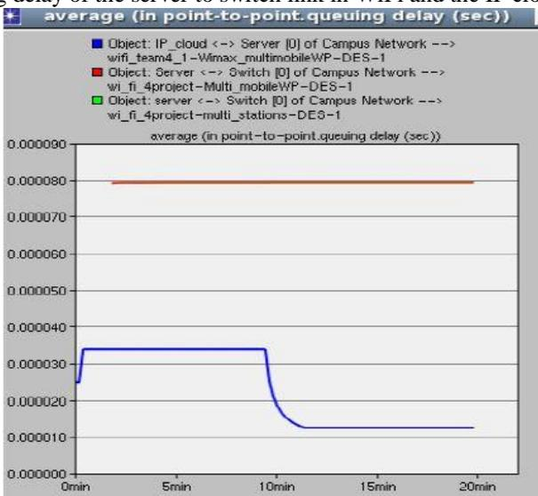
Figure 16: Average queuing delay of the switch to server link in WiFi and the IP cloud to server link in WiMAX.
