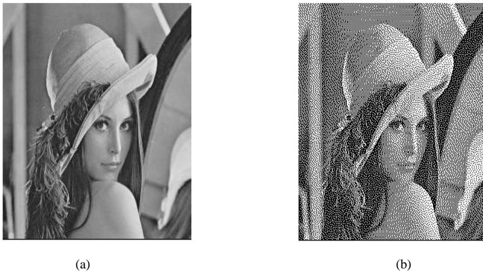
Fig 3: (a) The original image; (b) The halftoning image using Floyd and Steinberg Error filter algorithm
