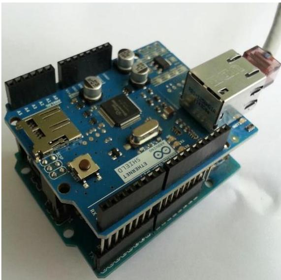
Fig. 10: Picture depicting the Arduino with Ethernet
