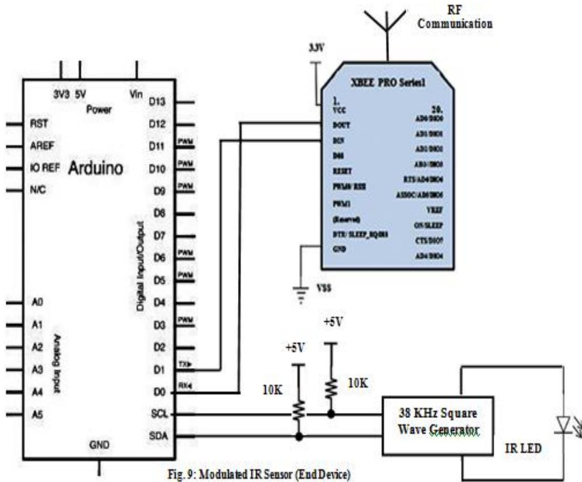
Fig. 9: Modulated IR Sensor (End Device)
