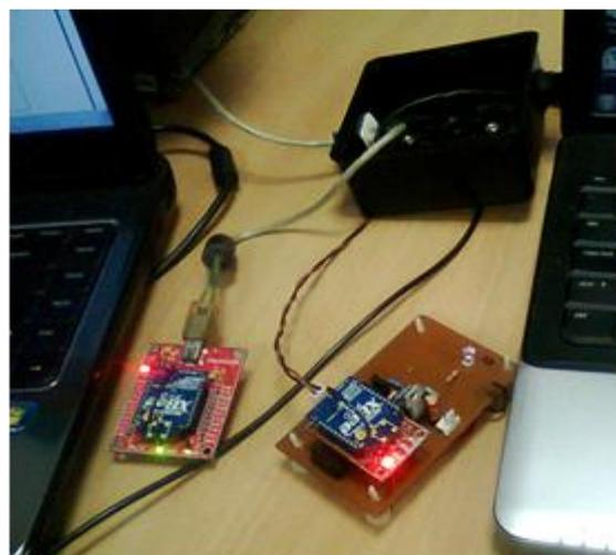
Fig. 13: Picture depicting the two XBees configured as end devices
