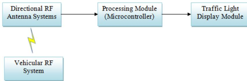
Fig. 2: Block diagram of Smart Traffic Light Control System (STLC)
