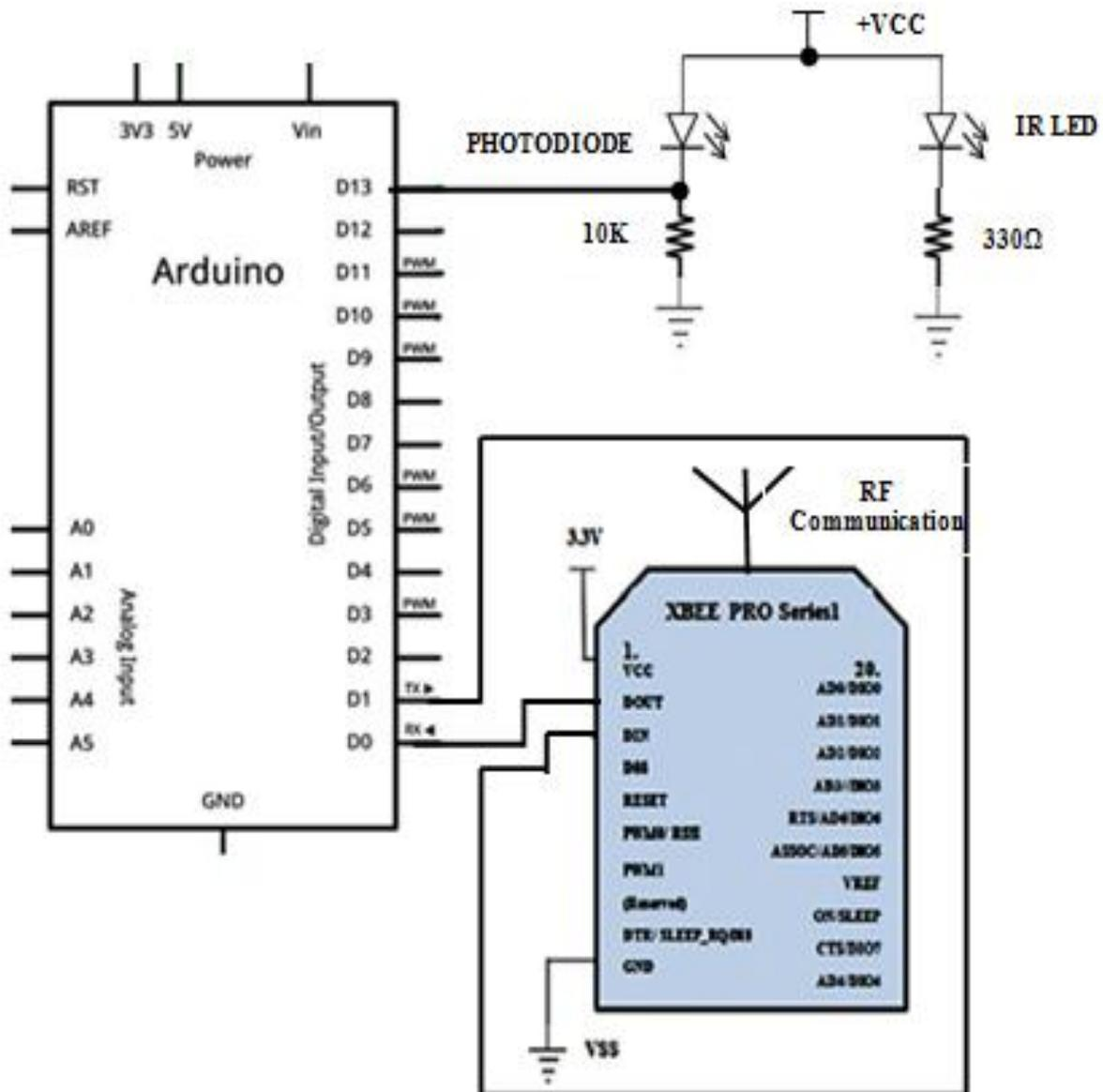
Fig. 8: Simple Proximity Sensor (End device)
