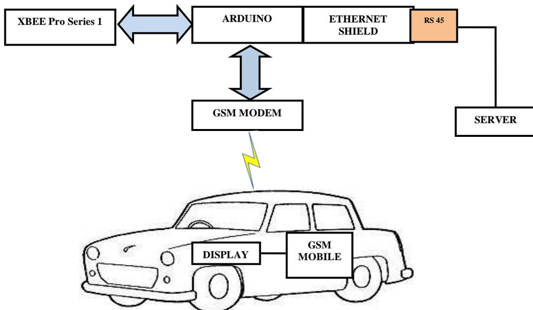
Fig. 6: Communication of Sensing System with Vehicular system for routing
