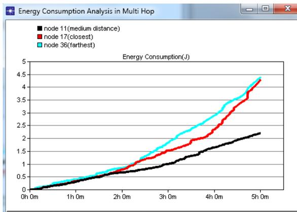
Figure 10: Energy consumption analysis in multi hop
