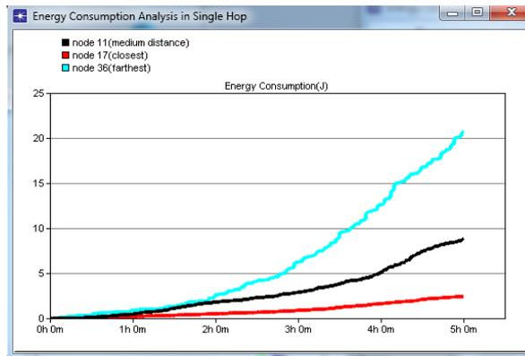
Figure 9: Energy consumption analysis in single hop
