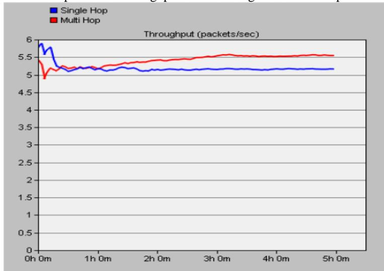
Figure 13: Farthest Distance Node Throughput
