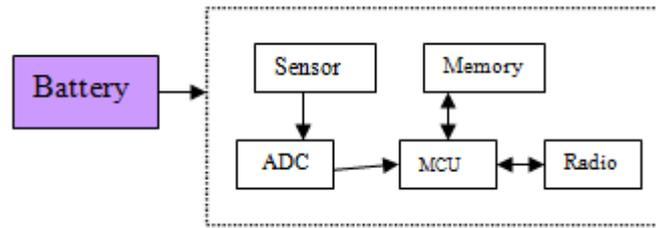
Figure 1: Wireless Sensor Network Architecture
