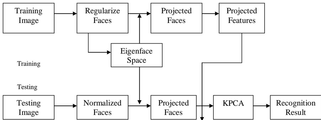
Fig.2. Model of KPCA face Recognition System
