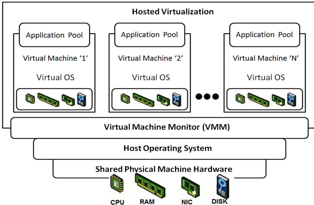
Fig. 1 Virtual Machine architecture for a server
