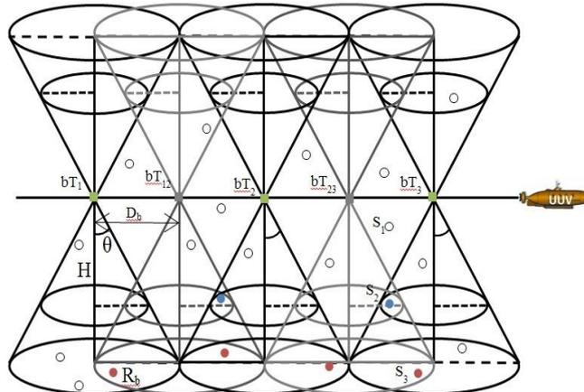
Fig. 3: 3D UW-ASN scenario involving the UUV, beacons and sensor nodes
