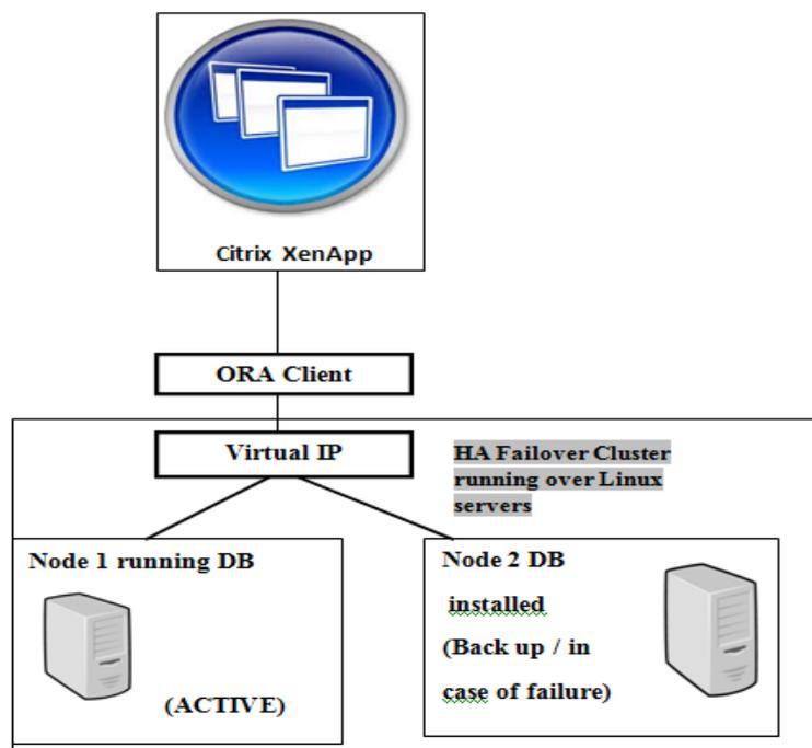
Figure4: Proposed Architecture preventing single point of failure
