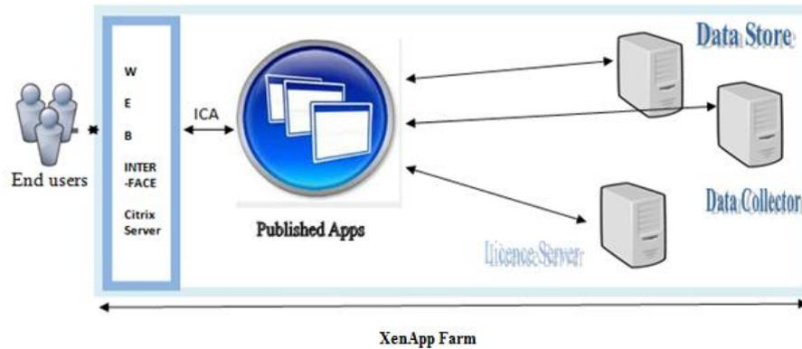
Figure 1: XenApp Server Architecture
