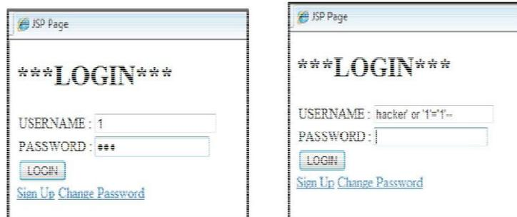
Figure 1: Example login – Normal case Figure, Figure 2: Example login – attack case
