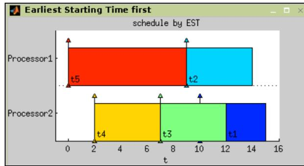
Figure 6. Earliest Starting time first Algorithm Gantt chart
