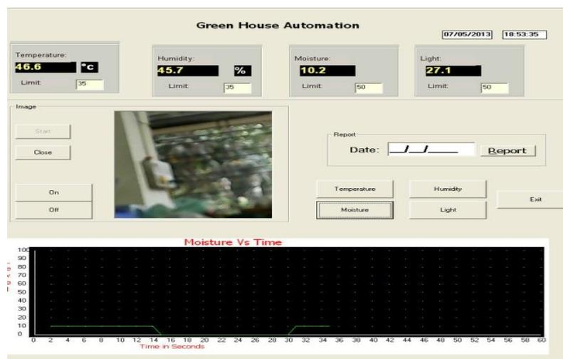
**Figure 4: Soil Moisture versus time**
